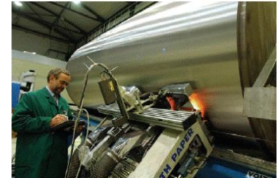
"Virtual Reference Grinding" of a paper dry drum
