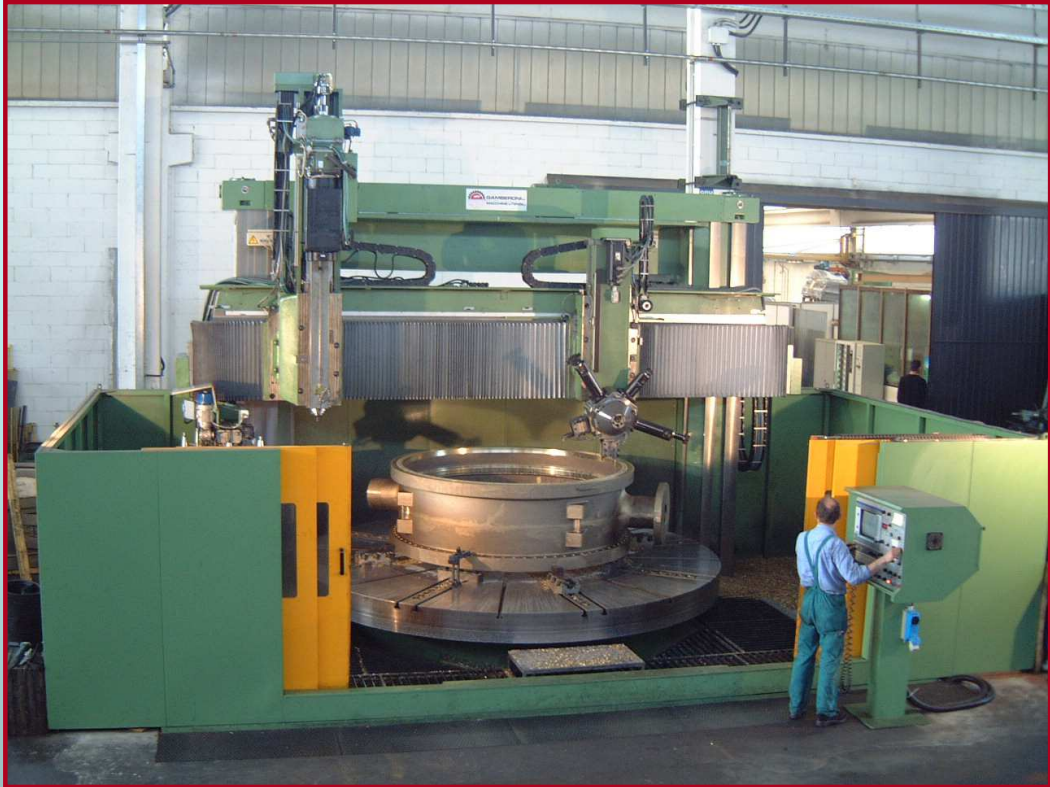
TITAN 4000 Vertical turning and drilling machining, capability up to DN 160" (4,000 mm.)
